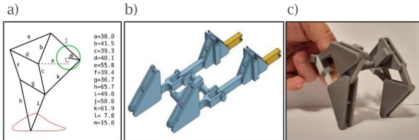
Fig. 1: The design activity, a Jansen’s leg structure a) structure and motion profile b) CAD model and c) printed prototype. Image from [1].
